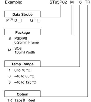
Note: 1. Data In strobed on rising edge of the clock (C) and Data Out synchronized from the falling edge of the clock.
